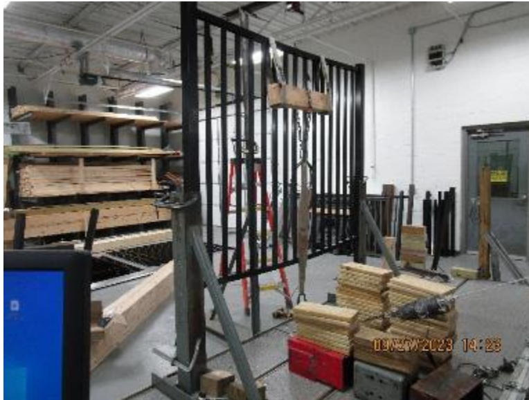
Photo No. 1 Method A Test on the 2-Rail System
